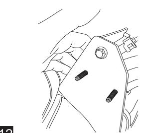
Set frame mount into position and tighten two bolts. Torque to 16 ft-lbs. Note: See step 1 for orientation on passenger side.
