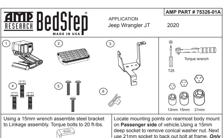
use 21mm socket to back out bolt at frame. Only remove enough to slide bracket into position.
