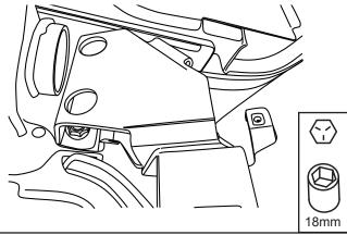
Replace brace and slide support strap over stud. Use supplied hardware to bolt strap to assembly. Torque to 41ft-lbs/ 55Nm.
