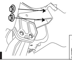
Insert threaded bracket into bumper and assemble bracket with supplied bolt. Use slotted end of bracket at bolt.
