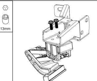
Torque Bolts to 33ft-lbs /44Nm.
