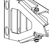
NOTE: If aftermarket hitch is installed, 2 bumper studs may need to be replaced. Recommended bolt size: M14x2.0x50 Class 10.9
