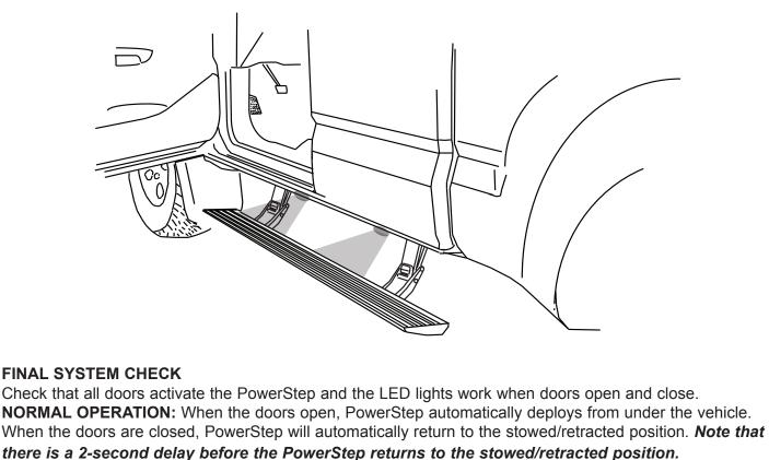
**CORRECT OPERATION OF LIGHTS:** All four lamps will illuminate upon opening any door of vehicle. Lamps will stay on until restowing of both Power Steps or until 5 minutes has expired with the doors open. When the lights timeout after 5 minutes, they can be reillumintated by closing and opening any door of vehicle.
