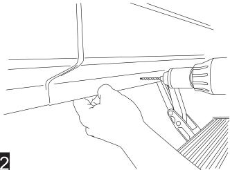
Insert grommet into drilled holes. Insert lamp wires through the grommets. (Silicon lube will help wires slip through grommets.
