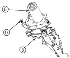
Install motor linkage on driver side in second set of factory running board holes from front. Use flange bolts (10) and torque to 22 ft-lbs / 30Nm.
