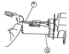
Slide rubber grommet on wire harness into slot of motor cover. Install motor cover onto motor.
