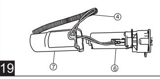
Partially separate the plastic rivet from the pin by bending the pin back and forth. Slide motor cover over motor and insert plastic push pin rivets in mounting holes of motor cover. Drive pin flush with rivet head. Use pliers to ease installation.
