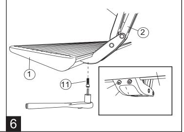
Repeat linkage installation on passenger side.
