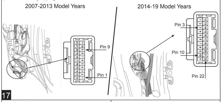
Insert plug from wire harness onto motor.
