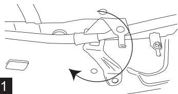
Secure parking brake cable support to frame so that the bolt is now below the cable.
