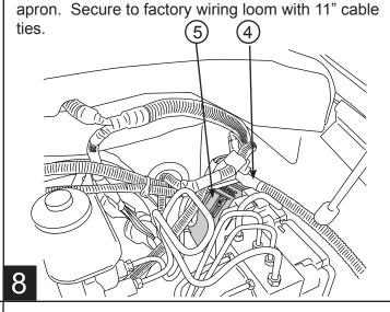
Install controller under hood on driver side fender
