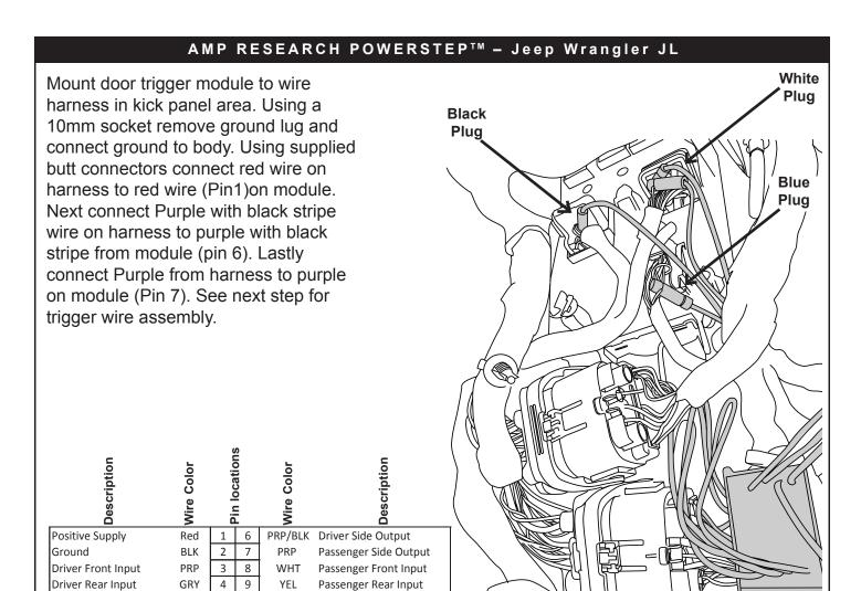
Locate the white connector panel against passenger side kick panel area. Locate three connectors as shown below and connect powerstep trigger wires as indicated in the chart. Match pin locations called out in previous step.
