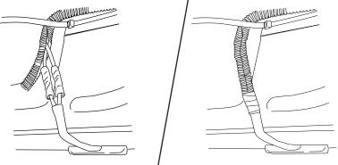
Reinstall Fuses from Powerstep Wire Harness.
