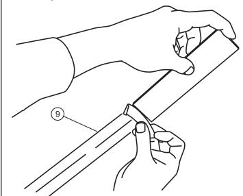
Slide 3 center tubes into the open ends of the bent tubes as shown. Insert center tube with logo into the center tube.
