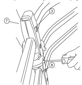
NOTE: Do not over tighten as this may strip out. Fastener will reach a noticable stopping point.
