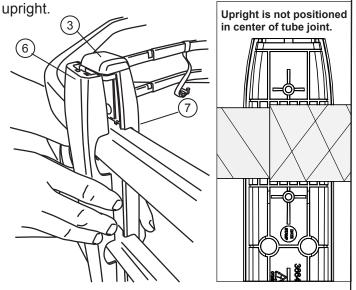
NOTE: The inside of the upright is stepped to fit correctly around the small and large diameter tubes.
