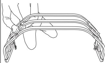
Note: Install Strap Buckle Assembly to center tube of Pivot Upright Assembly.
