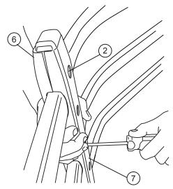
NOTE: Do not over tighten as this may strip out. Fastener will reach a noticable stopping point.
