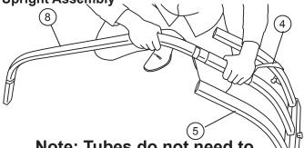
Note: Tubes do not need to be pushed in to taped edge.
