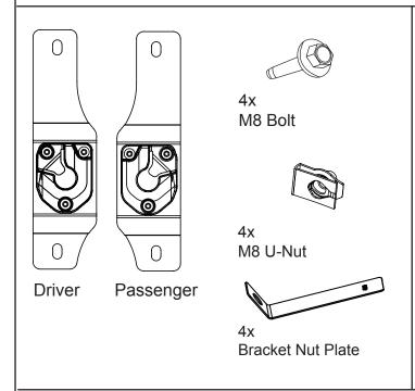
Assemble U-Nuts on to bracket plates in the orientation shown.
