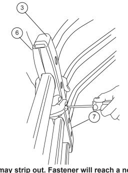
8 NOTE: Do not over tighten as this may strip out. Fastener will reach a noticeable stopping point.
