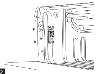
Place Mounting Bracket aligned with top hole. Allow bracket to hang vertically. Mark (Center Punch) location of lower hole using the bracket slot as a template. Remove bracket. Drill hole with 1/8" drill bit then drill out hole with 21/64" drill bit. Use file to remove burrs. Apply primer to edge of hole. Allow primer to dry.
