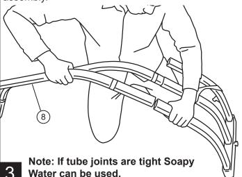
Insert the bottom long tube into the bottom tube of the 3-tube assembly.
