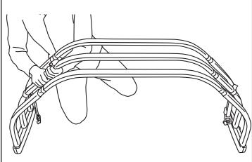
Note: Install Strap Buckle Assembly to center tube of Pivot Upright Assembly.
