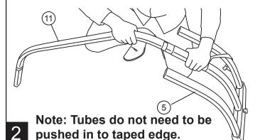
Insert the top long tube into the top tube of the 3-tube assembly.
