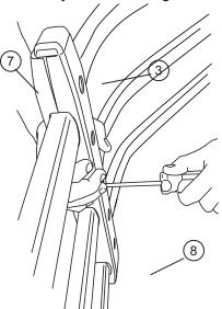
NOTE: Do not over tighten as this may strip out. Fastener will reach a noticable stopping point.
