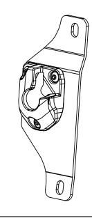
Use the M5 bolts and nuts to fasten the Quick Mount Bracket to the mounting bracket. Apply thread locker to the tip of the M5 bolt. Torque to 8 ft. lbs. Allow 10 minutes to dry before handling. (Passenger side shown)
