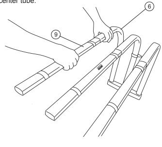
Connect the two halves. Make sure there is at least 3" overlap with the bent tubes on each side.
