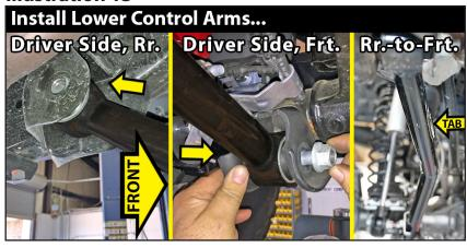
mounts using the factory hardware with the bolt pointing inward. [21mm & 24mm]
