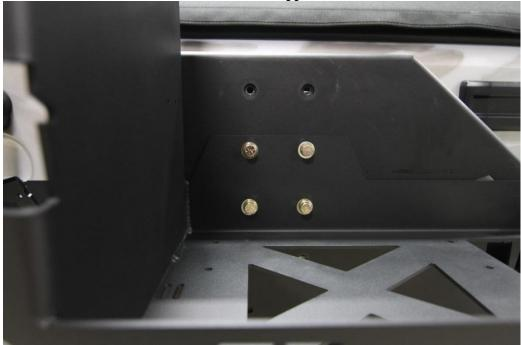
Note: Some older versions of tire carriers may not have the necessary hole to attach the  $5^{th}$  mounting bolt to the tray and cooler mount. This hole must be drilled out using a  $\frac{1}{2}$ " drill bit. It is recommend that you center punch the location then removed the cooler mount before drilling.
