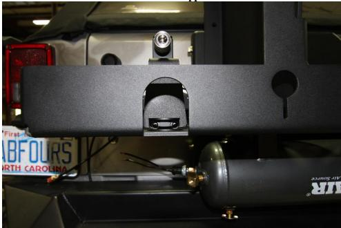
Figure 3: Pressure Gauge Bracket and 6-Port Block
