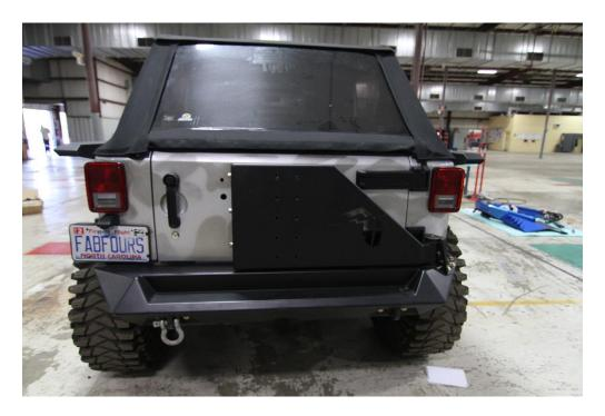
**2.** Using the provided 7/16 hardware, attach your cooler/compressor mount to the tire carrier.
