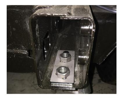
13. With a friend, carefully hold the bumper and swing arm assembly up to the Jeep and use the  $\frac{1}{2}$ " bolts to attach the nut plate along with the OEM side bolts.
