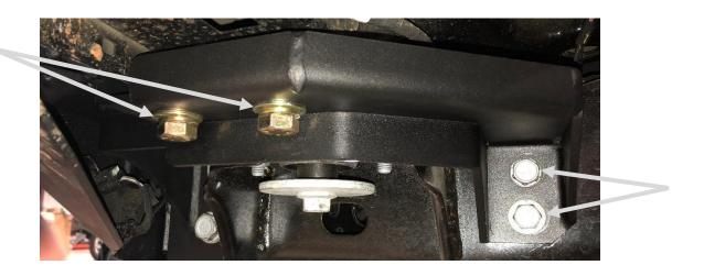
15. Take the turn buckles and put them through the swing arm and attach them using the <sup>1</sup>/<sub>2</sub>" bolts with spacers and washers. (Tighten securely)
