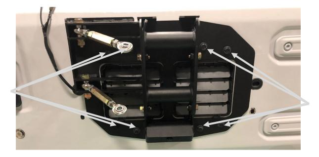
6. Take the rubber stops and attach them to the swing arm using the 3/8" bolts. (Make sure to push the stops up against the metal gussets as shown before fastening)
